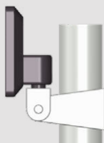
Round tube Ø 48 mm Connection from below
