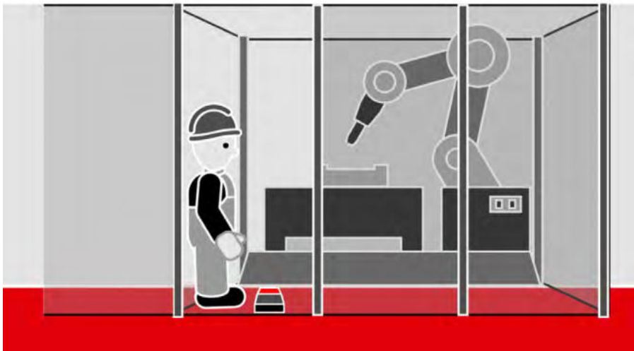
Teaching a robot function through a three-stage enabling footswitch
